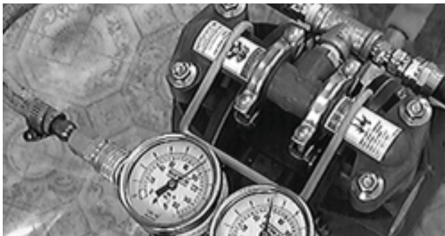
Figure 5. Proper pressure settings insure smooth spraying of 3500SI spray.
