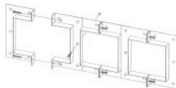
Fit cables into the bottom of the FCW-44; close the lid and slide the FCW-44 into the opening leave 28.6 mm (1-1/8 in.) between FCWs
